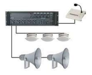
Public Address System (PA system) is an electronic sound amplification and distribution system with a microphone, amplifier and loudspeakers, used to allow a person to address a large public, for example for announcements of movements at large and noisy air and rail terminals.
