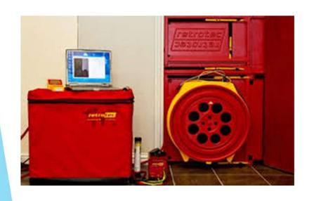
An Integrity test predicts how long fire suppressant agents take to descend to a given level in the room without having to release the agent itself. The Integrity test is carried out using: • Modular adjustable panels for the door frame which adjusts to fit a wide variety of door sizes
